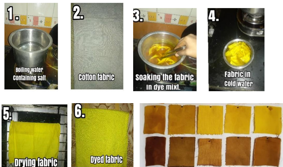
Figure 3 Dyeing of cotton fabric (picture 1 to 4); drying of cotton fabric (5 & 6) and different shades of curcumin with mordant dyeing.
