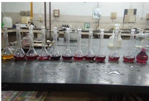
Picture (a): 100 cm 3 standard measuring flasks containing different ppm concentration of fluorides ions solution for calibration curve.
