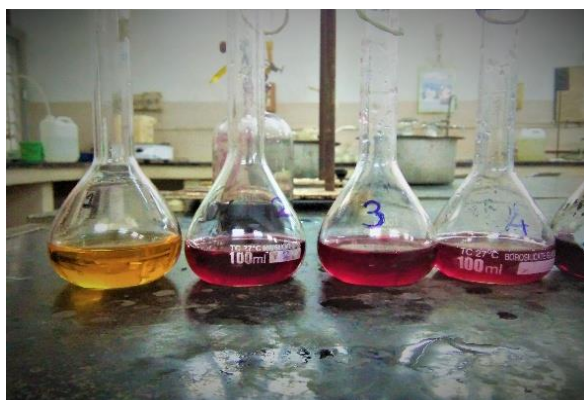
Picture (b): 100 cm 3 standard measuring flasks of various water sample containing unknown amount of fluorides ions
