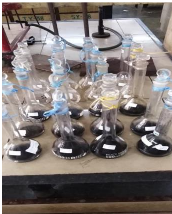
Picture (b): 100 cm 3 standard measuring flasks with adsorbent and fluoride solution before dilution
